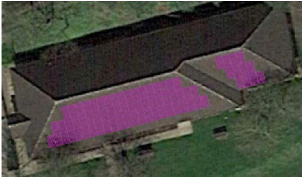
Figure 3 – Proposed location of solar panels for a 20kWp on the roof of the Pavilion
