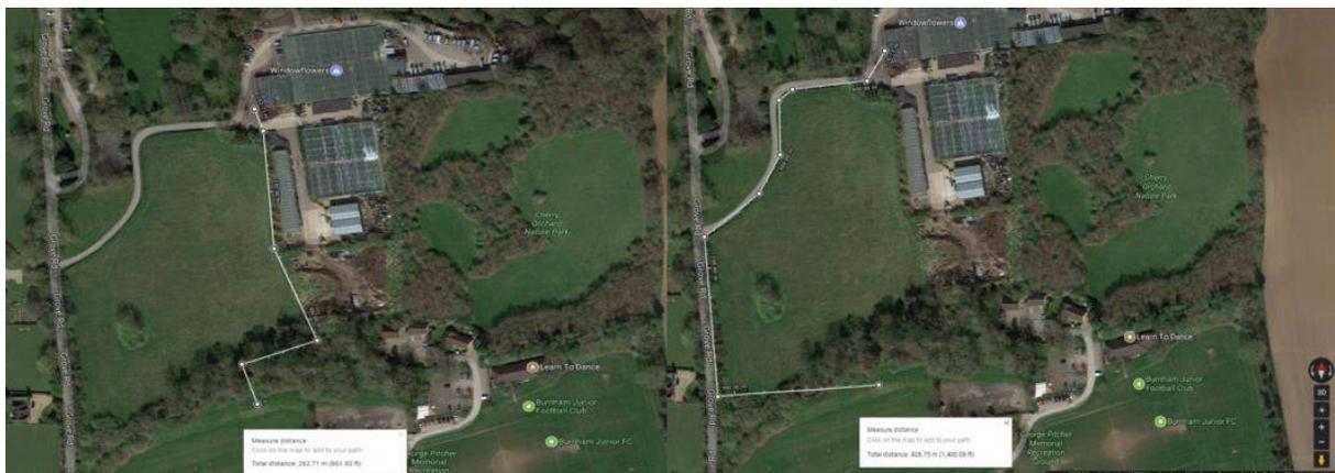
Figure 6 – the routing options considered for the installation of a private wire
